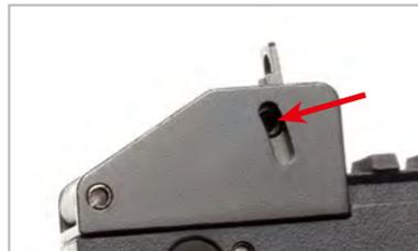
Adjust the sight horizontally by turning windage adjusting screw clockwise and counterclockwise to shift the rear sight to right and left respectively.
