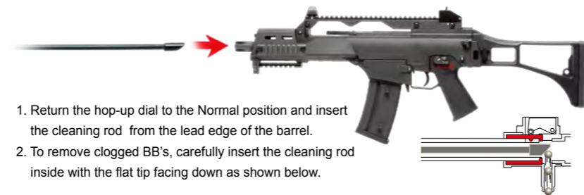
1. Return the hop-up dial to the Normal position and insert the cleaning rod from the lead edge of the barrel.
