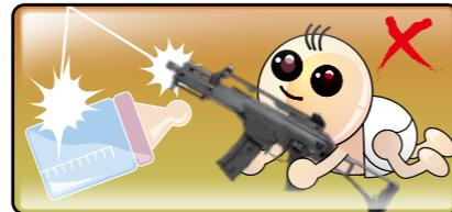
Always attach the safety cap to the muzzle, remove the battery and store the air gun in a case or bag and at a place that is out of reach of children.
