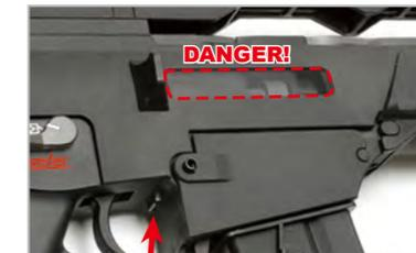
Press the bolt catch lever to release the bolt.
