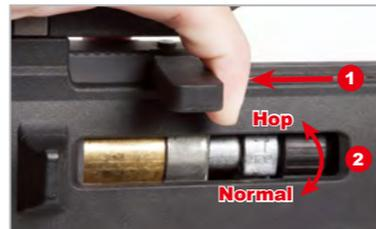
1. Pulling the charging handle backward will open and lock the bolt.
