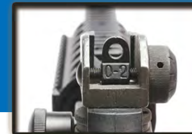
COMMON SHOOTING Used for full automatic firing.
