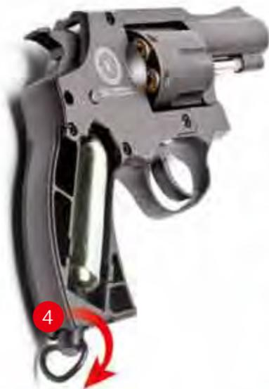
4. Turn the puncture screw clockwise to puncture the CO2 cartridge.
