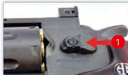
1. Push and hold the selector to the "OPEN" position.
