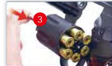
3. Push the ejector rod to unload the brass shells.
