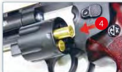
4. Insert six brass shells into the cylinder.
