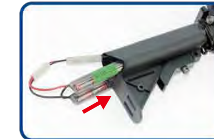
Insert the battery into stock.
