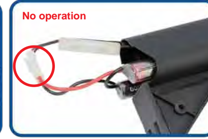
Check the battery and connector.
