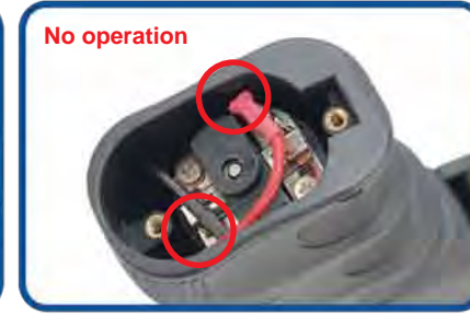
Check the wire set contact with motor.
