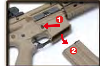
Remove the magazine.
