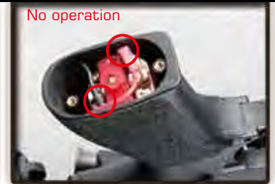
Check the wire set contact with motor.
