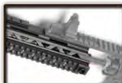
Reinstall the Q.D. rail system.
