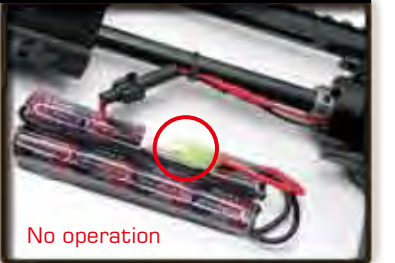
Check the battery and connector.
